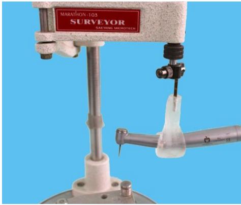
Figure 3 – Airtor handpiece attached to the surveyor using custom made device
